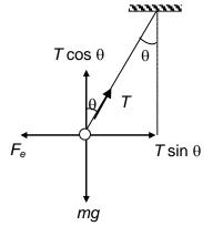
Since the sphere is in equilibrium, the resultants of the forces in the horizontal and vertical directions must separately add up to zero. thus
